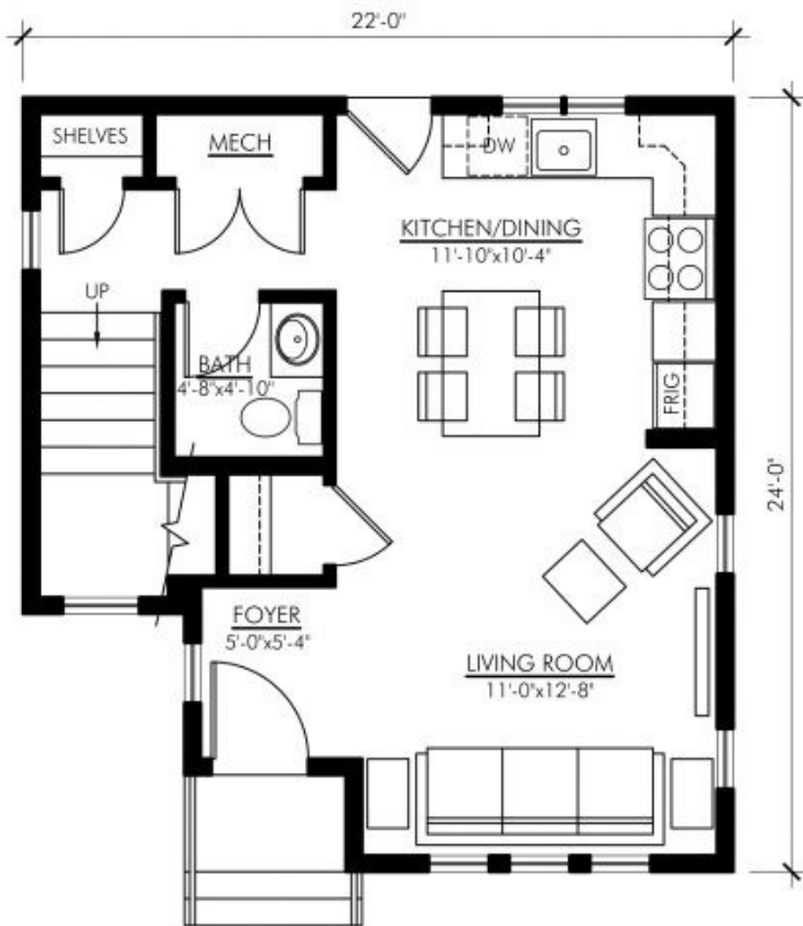
MAIN FLOOR PLAN - 473 SQ FT AUSTRING - 946
